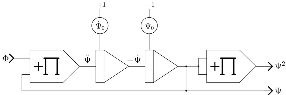
Figure 1: Setup for the one-dimensional SCHRÖDINGER equation
