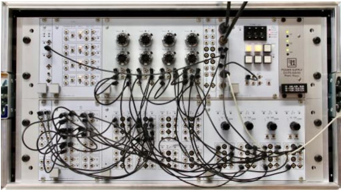
Figure 2: Setup of the ballistic trajectory problem on an Analog Paradigm Model-1 analog computer
