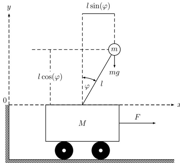
Figure 1: Configuration of the inverted pendulum
