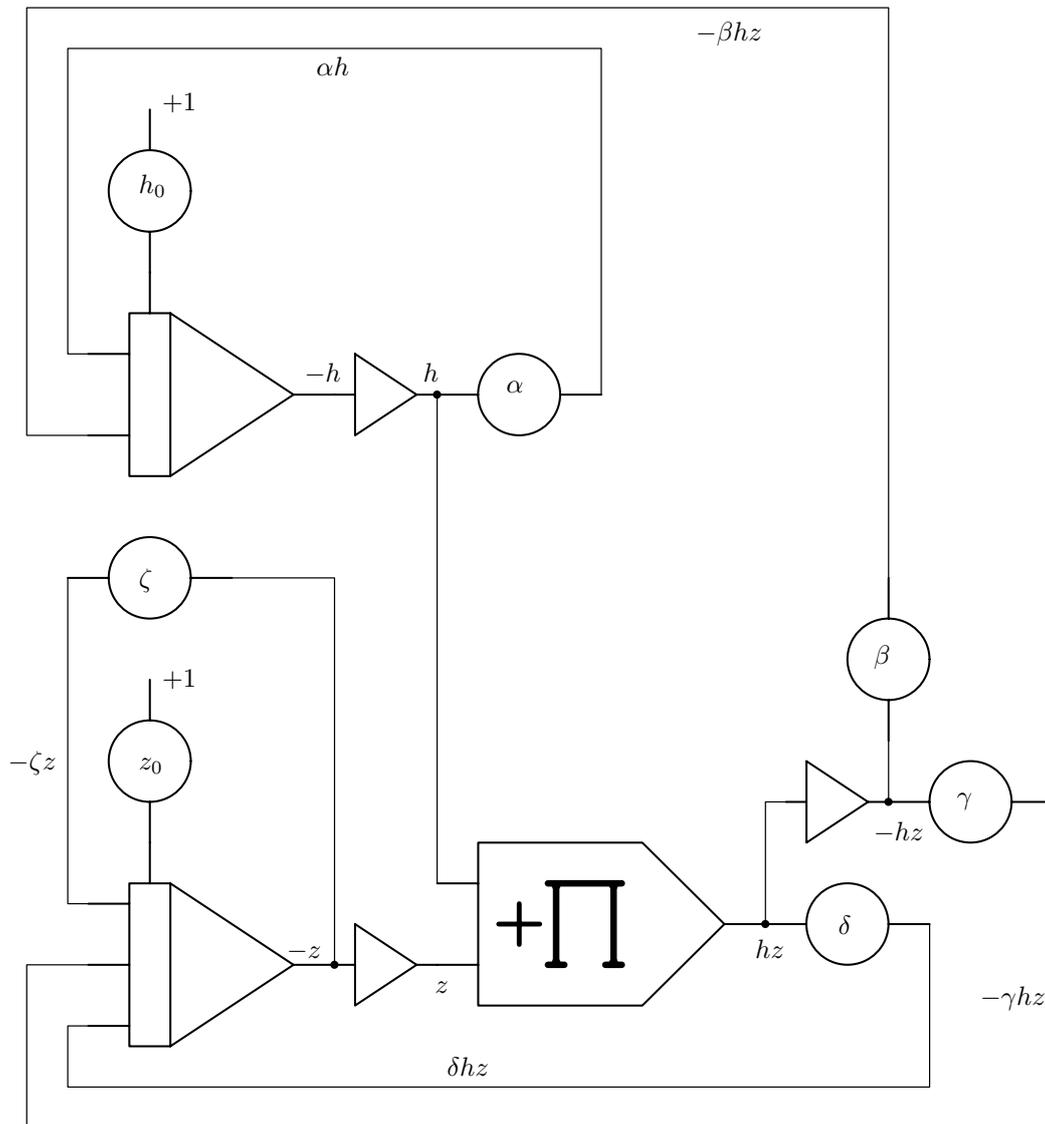
Figure 1: Analog computer program for equations (1) and (2)
