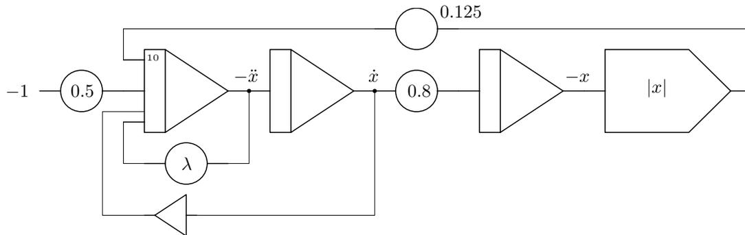
Figure 1: Computer setup for nonlinear chaos
